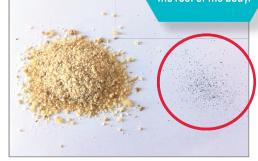
Pass a magnet underneath the paper. Small flecks will start to separate from the crumbs, attracted to the magnet. This is the iron that was added to your cereal.
