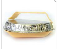
Holding the handle, put the pie tin on the box for 15 seconds. Build up more charge by repeating steps 4–6.
