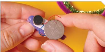
Carefully position the battery over the negative wire and press it down firmly, making sure that you leave the red wire loose. Then, cut two lengths of pipe cleaner and stick them down between the battery and motor.
