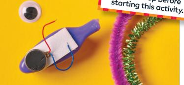
peel off the other piece of backing tape and stick the vibration motor to the front of the toothbrush head. Then stick the negative wire (black or blue coloured) down on the sticky foam pad.
