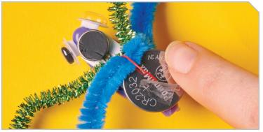
Attach googly eyes to the sides of the brush head using small pieces of foam pad. To make your bristle bot go, press the red wire down onto the top of the battery and hold it in place with a small piece of tape.
