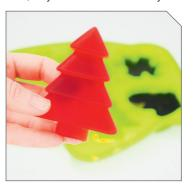
Leave to set in the moulds for five days, then remove. Allow the bioplastic shapes to harden for two more days out of the moulds.
