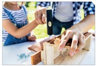
It's time to start constructing. Using a hammer and nails, carefully assemble the bird box. Add a side panel to the back first, and then fit the floor. Finally attach the other side panel.
