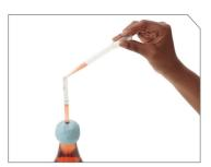
Add liquid into the straw using the dropper. Continue until the liquid is level with one of your marks.
