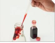
Fill the bottle with spirit and add a few drops of food colouring. Suck up some liquid using the dropper.
