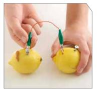
Link the coin on one lemon to the nail on the next, using an electrical connector. Continue until you have connected all five lemons together.
